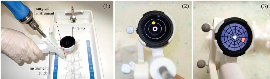
**Fig. 1.** (1) Hand-held navigation device, green line: instrument trajectory, red line: target trajectory, (2) Close view of Circle Display, (3) Close view of Grid Display (Color figure online)
